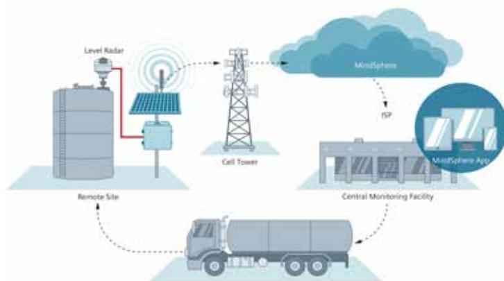
Siemens remote tank monitoring puts tank data at your fingertips with secure wireless communications, an extensive instrumentation portfolio and MindSphere.
